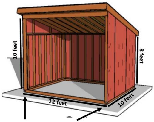
Four 4x4 corner posts in 3 feet of concrete below grade
