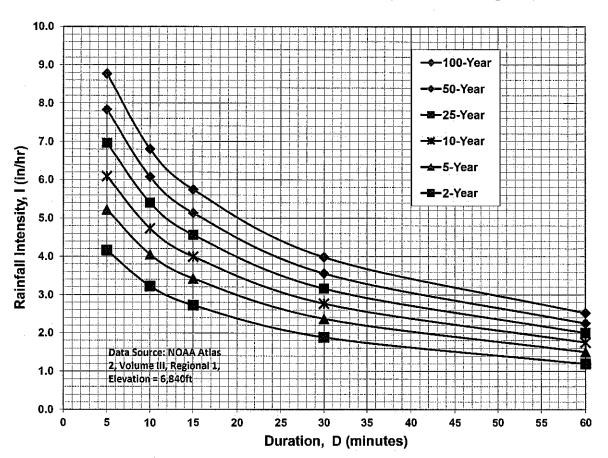
Figure 6-5. Colorado Springs Rainfall Intensity Duration Frequency
