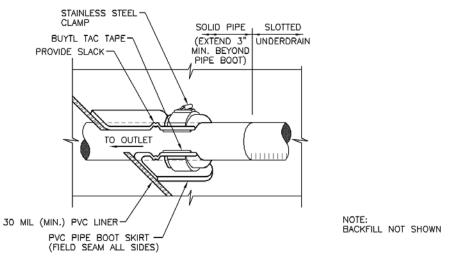
Figure B-2. Geomembrane Liner/Underdrain Penetration Detail
