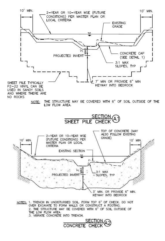
Figure 9-27. Check structure details (Part 2 of 3)
