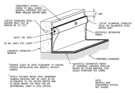
Figure B-3. Geomembrane Liner/Concrete Connection Detail
