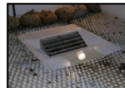
CDOT Type D Inlet Parallel (30° Incline & Depressed)
