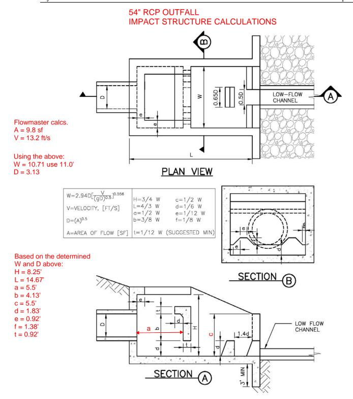
Figure 9-45. UDFCD modified USBR type VI impacts stilling basin (general design dimensions)
