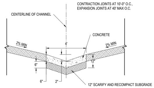
**CONCRETE TRICKLE CHANNEL DETAIL**
