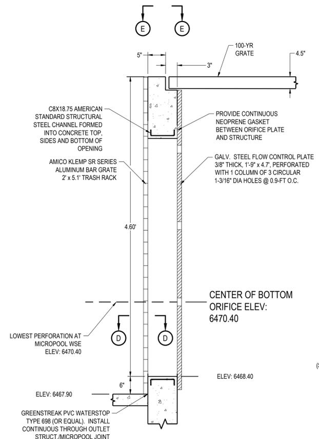
**OUTLET STRUCTURE - SECTION C-C**
