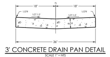
3' CONCRETE DRAIN PAN DETAIL
