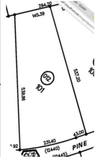
The barn will be setback 15ft on the left border, 100 ft on the right border, 115 ft from the back border and 385 ft from the front border. Property dimensions (insert on right); Left: 539.96 ft, Right: 537.20 ft, Back: 145.39 ft, Front: 231.40 ft + 43 ft
