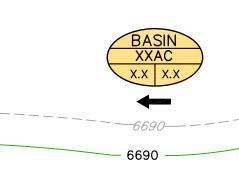
BASIN I.D. ACREAGE 5 YR/100 YR CFS DIRECTION OF FLOW EXISTING CONTOUR PROPOSED CONTOUR
