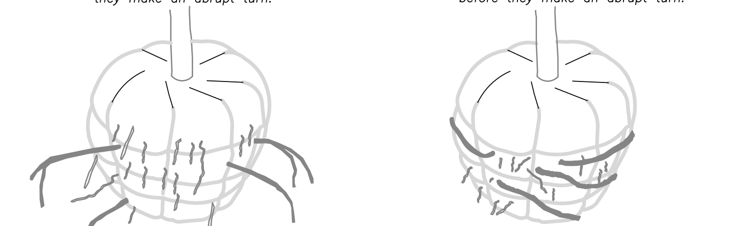
Remove structural roots (4 shown in black) extending from root ball.
