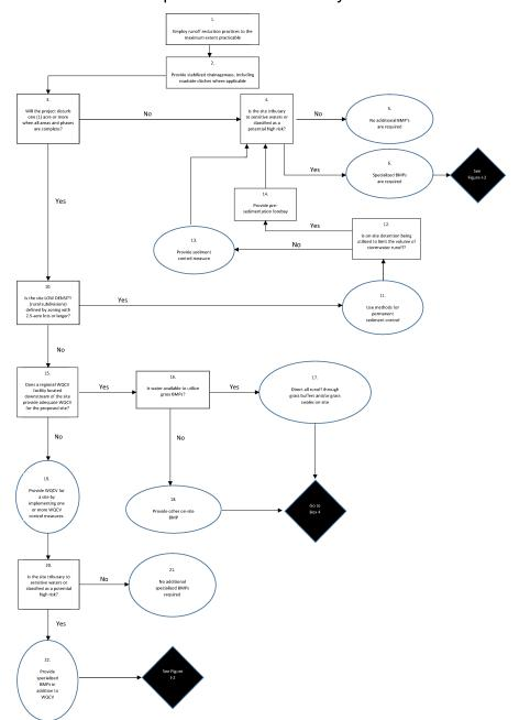
Figure I-2. BMP Requirements Flowchart for New Development and Redevelopment Sites—For Selecting Post-Construction BMPs in Compliance with El Paso County's Stormwater NPDES Permit
