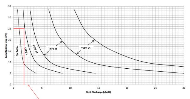
**Figure 12-21. Embankment protection details and rock sizing chart** (adapted from Arapahoe County) 107.7 cfs/60 ft = 1.80
