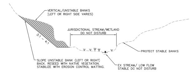
CHANNEL CROSS— SECTIONS PROPOSED STABILIZATION N.T.S
