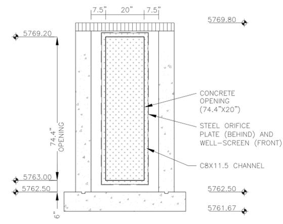
OUTLET STRUCTURE DETAIL - SECTION B-B
