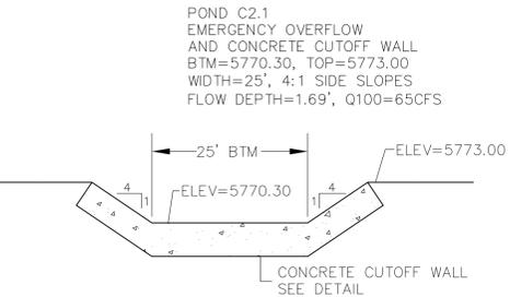
**POND C2.1 EMERGENCY OVERFLOW AND CONCRETE CUTOFF WALL PROFILE**
