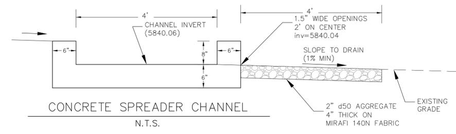
CONCRETE SPREADER CHANNEL
