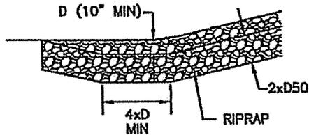
TERMINATION OF RIPRAP LINED SLOPE DRAIN
