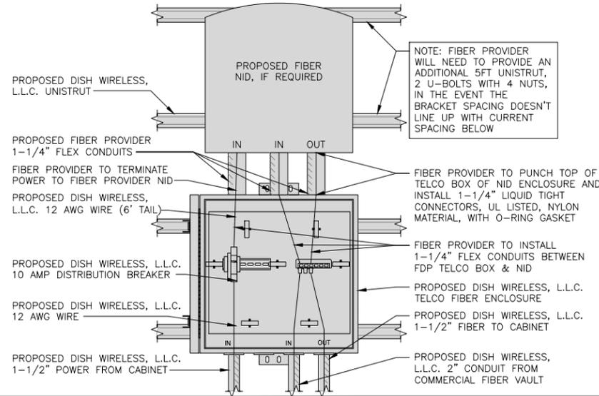
NOTE: FIBER PROVIDER WILL NEED TO PROVIDE AN ADDITIONAL 5FT UNISTRUT, 2 U-BOLTS WITH 4 NUTS, IN THE EVENT THE BRACKET SPACING DOESN'T LINE UP WITH CURRENT SPACING BELOW
