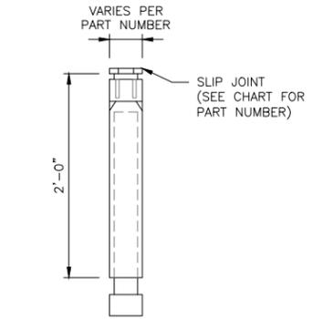
NOTE: CONTRACTOR TO INSTALL EXPANSION FITTING SLIP JOINT AT METER CENTER CONDUIT TERMINATION, AS PER LOCAL UTILITY POLICY, ORDINANCE AND/OR SPECIFIED REQUIREMENT.
