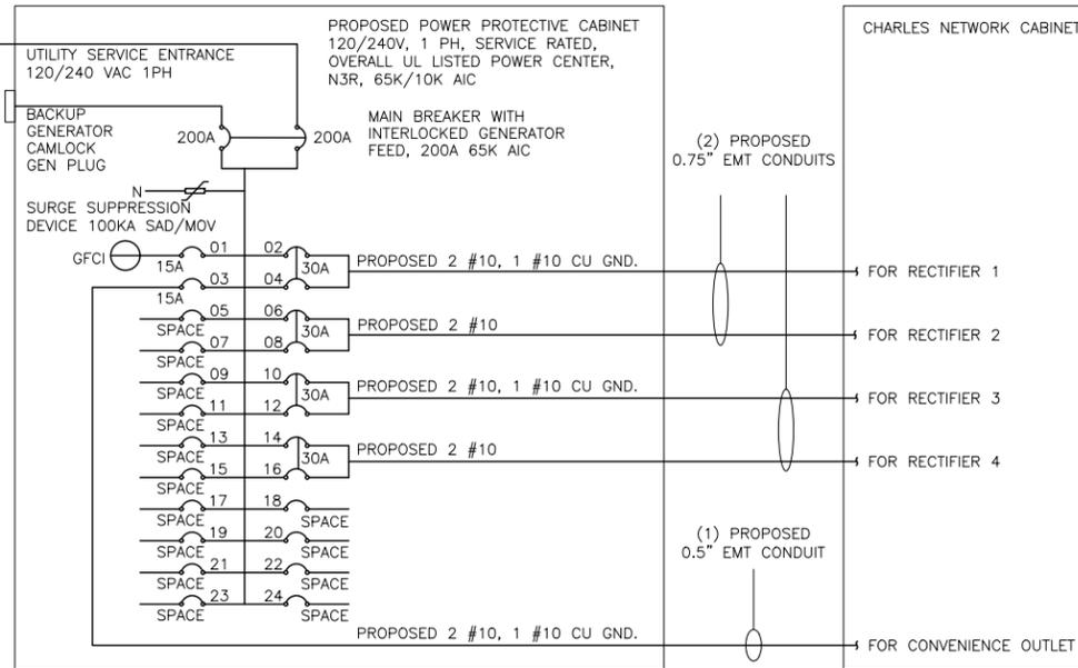
NOTE: BRANCH CIRCUIT WIRING SUPPLYING RECTIFIERS ARE TO BE RATED UL1015, 105°C, 600V, AND PVC INSULATED, IN THE SIZES SHOWN IN THE ONE-LINE DIAGRAM. CONTRACTOR MAY SUBSTITUTE UL1015 WIRE FOR THWN-2 FOR CONVENIENCE OUTLET BRANCH CIRCUIT.
