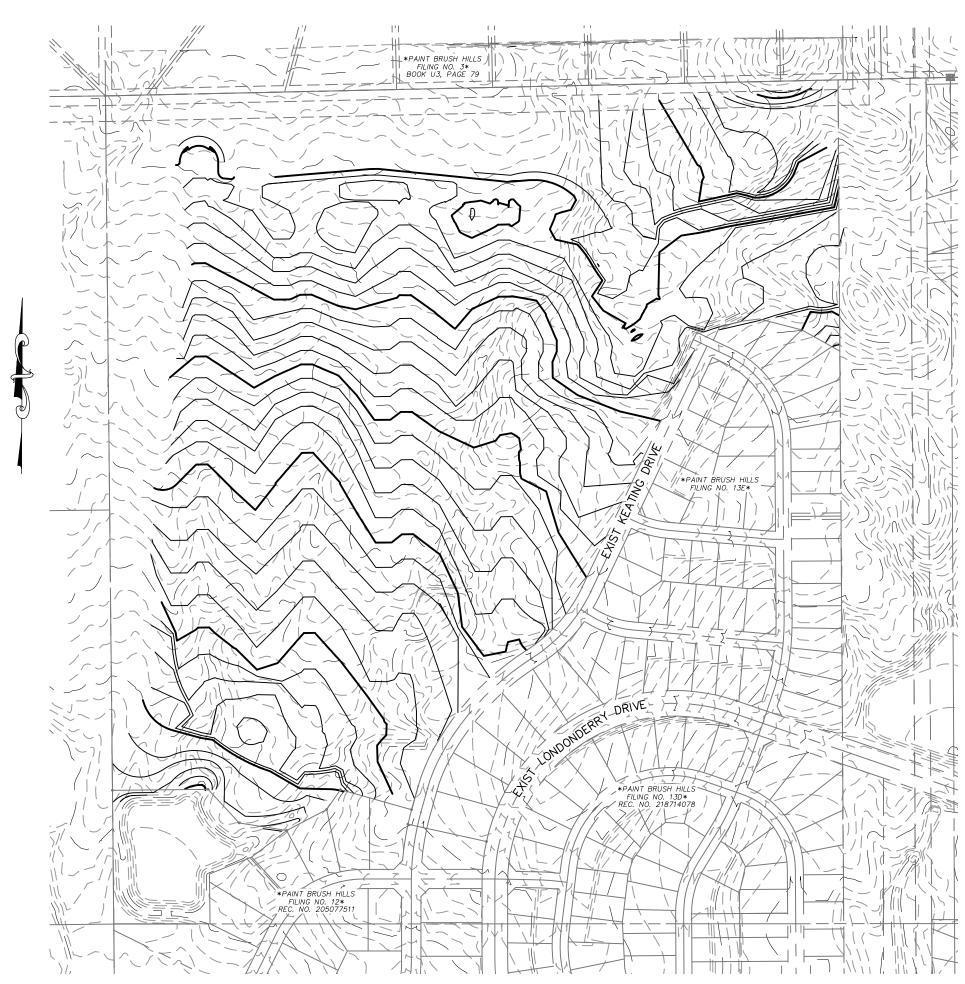
THE EROSION CONTROL DELINEATED ON THIS PLAN SHALL BE REGULARLY UPDATED BY THE CONTRACTOR. TEMPORARY SEDIMENT TRAP LOCATIONS WILL BE DETERMINED BY THE CONTRACTOR IN THE FIELD. EXISTING SITE TERRIAN GENERALLY SLOPES FROM NORTH TO SOUTHWEST AT GRADE RATES THAT VARY BETWEEN 2%
