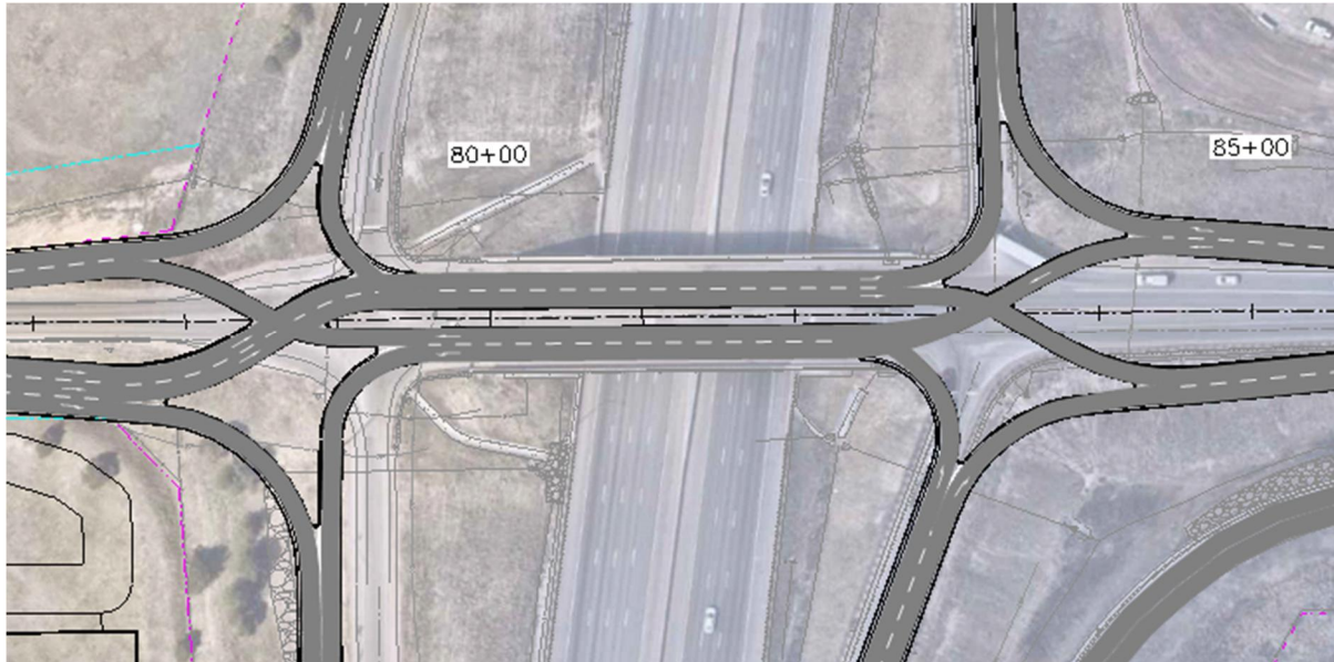
Figure 6 – County Line Road & I-25 Diverging Diamond Interchange Configuration
