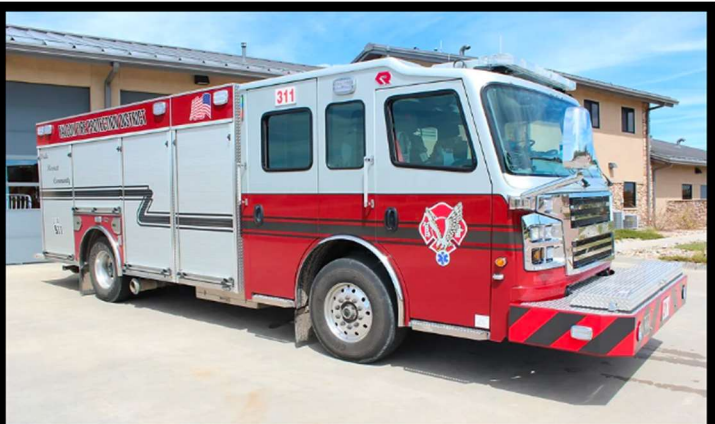
Engine 311 | 2018 Rosenbauer Commander | 1000 GPM Pump | 750 Gallons
