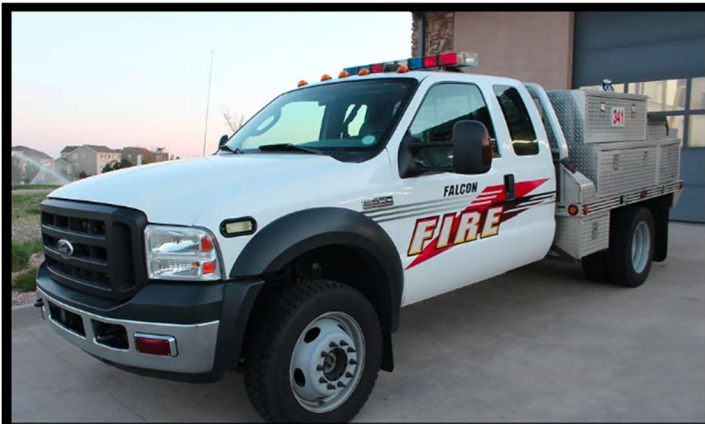
Brush 341 | 2005 Ford F350 | 50 GPM Pump | 300 Gallons
