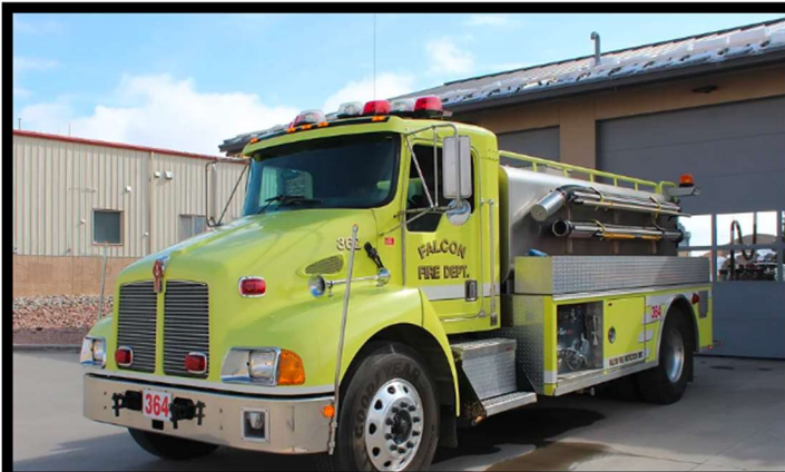
Tender 361 | 2001 Kenworth | 500 GPM Pump | 2000 Gallons
