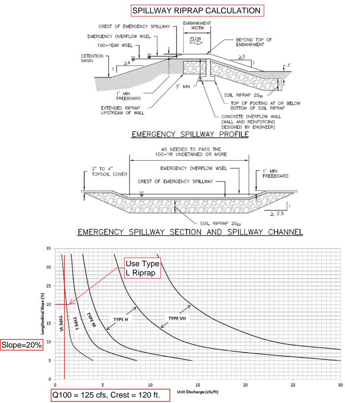
Figure 12-21. Embankment protection details and rock sizing chart (adapted from Arapahoe County)
