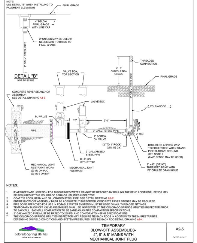
**TEMPORARY BLOW-OFF ASSEMBLIES- 4", 6" & 8" MAINS WITH MECHANICAL JOINT PLUG**
