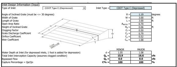
Warning 01: Sideslope steepness exceeds USDCM Volume I recommendation Warning 02: Depth (d) exceeds USDCM Volume I recommendation.
