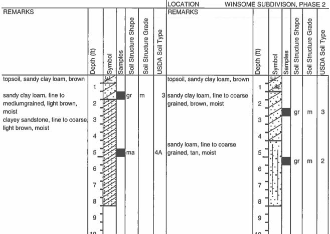
Soil Structure Shape granular - gr platy - pl blocky - bl prismatic - pr single grain - sg massive - ma
