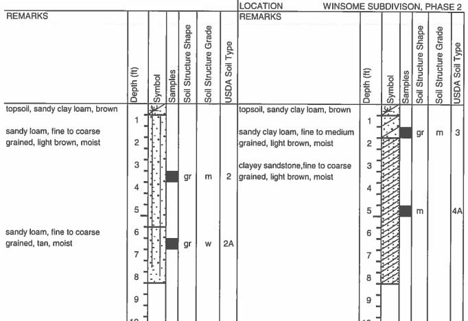
Soil Structure Shape granular - gr platy - pl blocky - bl prismatic - pr single grain - sg massive - ma Soil Structure Grade weak - w moderate - m strong - s
