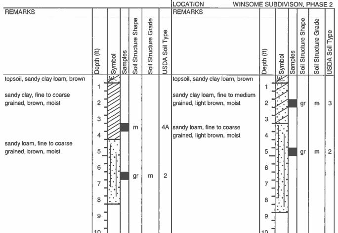
Soil Structure Shape granular - gr platy - pl blocky - bl prismatic - pr single grain - sg massive - ma Soil Structure Grade weak - w moderate - m strong - s loose - l
