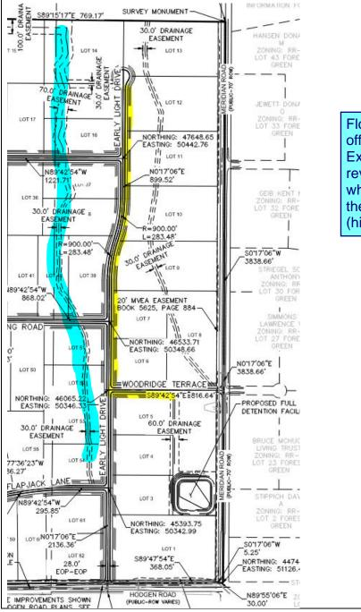
Flow from Pond 6 is primarily from off site flow and commercial lot. Explain why the design could not be revised to continue it's historic path which is the natural drainage way on the west side of early light drive (highlighted in blue)
