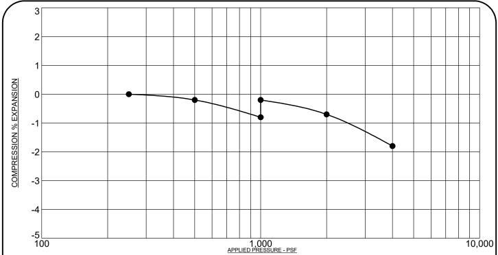
PROJECT: Copper Chase at Sterling Ranch, Filing No. 1, El Paso County, Colorado SAMPLE DESCRIPTION: CLAYEY SANDSTONE NOTE: SAMPLE WAS INUNDATED WITH WATER AT 1,000 PSF
