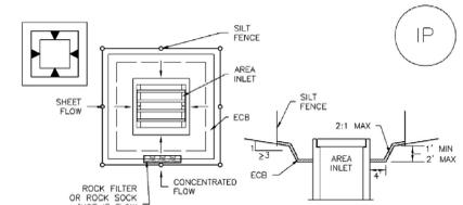
**OVEREXCAVATION INLET PROTECTION INSTALLATION NOTES**
