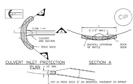
**CULVERT INLET PROTECTION INSTALLATION NOTES**
