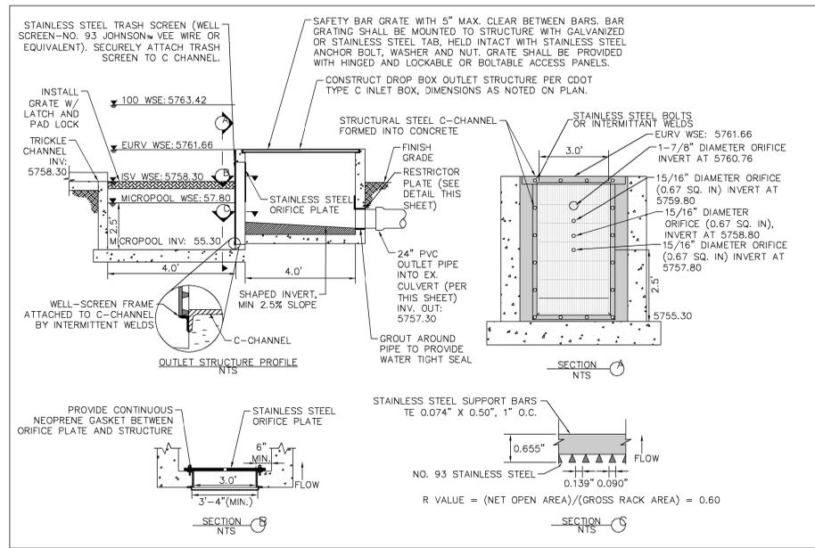
**OUTLET STRUCTURE PROFILE DETAIL**
