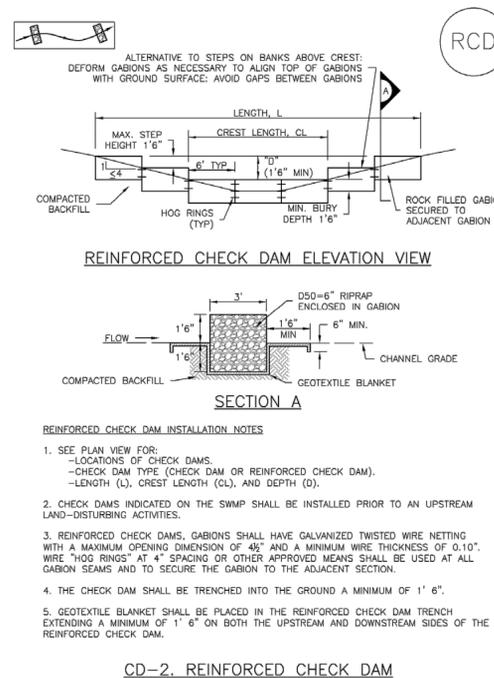
REINFORCED CHECK DAM ELEVATION VIEW
