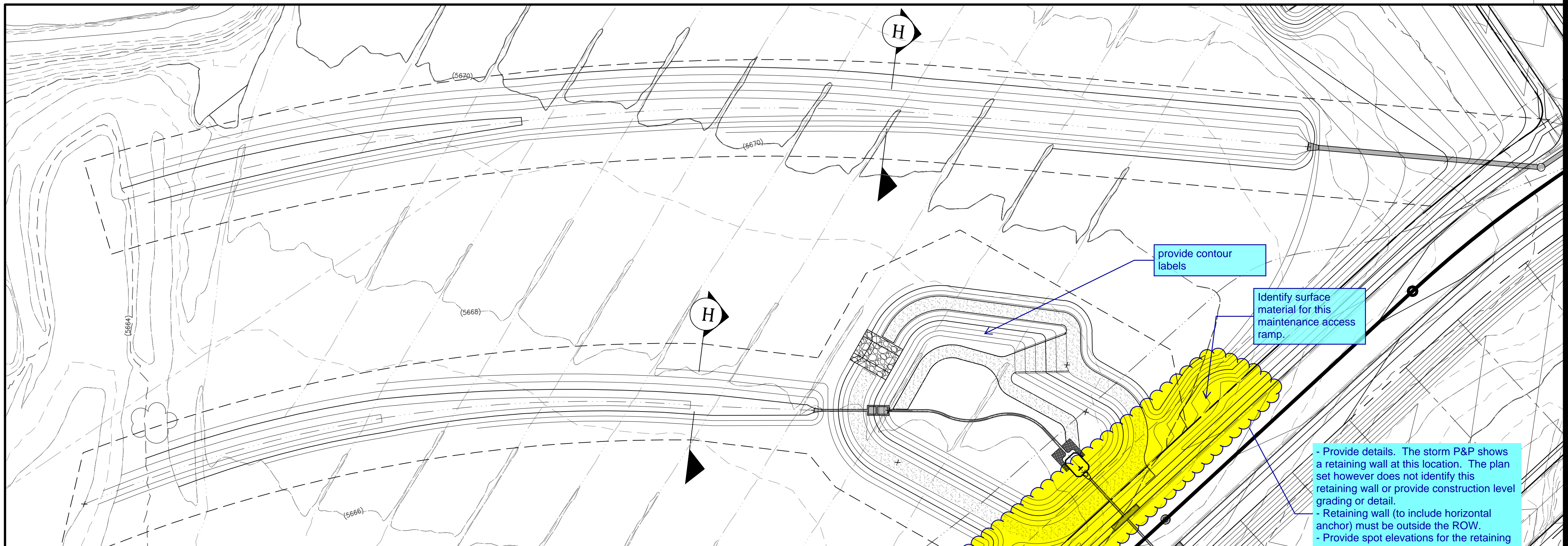
EXTENDED DETENTION BASIN 'A' AND GRASS-LINED CHANNELS TO WEST FORK JIMMY CAMP CREEK
