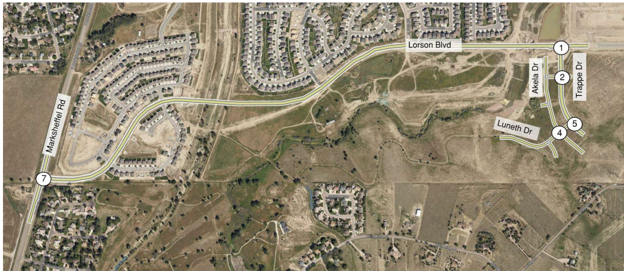
Figure 8. Creekside at Lorson Ranch Filing No.2 Project Trips (AM Peak Hour)
