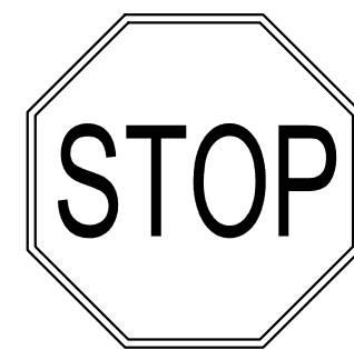
30"x30" MINIMUM SIZE BACKGROUND 4090 (3M-WHITE DIAMOND GRADE) OR EQUIVALENT FOREGROUND 1172 C (3M-RED EC FILM) OR EQUIVALENT
