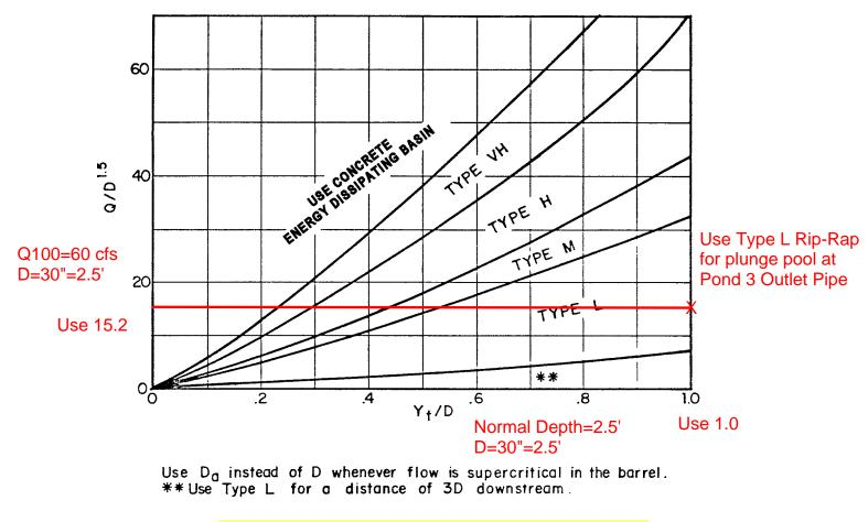
Rip-Rap sizing for Plunge Pool at Pond 3 Outlet Pipe
