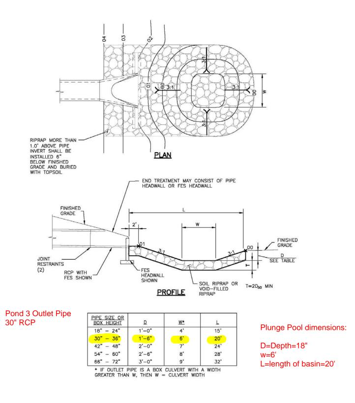
Figure 9-37. Low tailwater riprap basin
