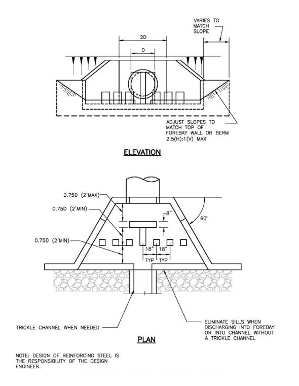
Figure 9-43. Modified impact stilling basin for conduits 18" to 48" in diameter (Part 1 of 2)
