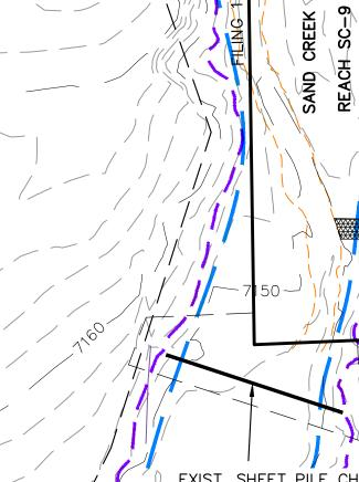
EXIST. SHEET PILE CHECK STRUCTURE W/ CONC. CAP
