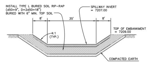
**EMERGENCY SPILLWAY CROSS SECTION**
