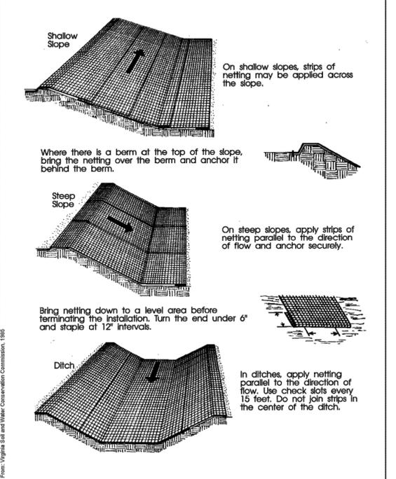
City of Colorado Springs Storm Water Quality Figure ECB-1 Erosion Control Blanket Application Examples
