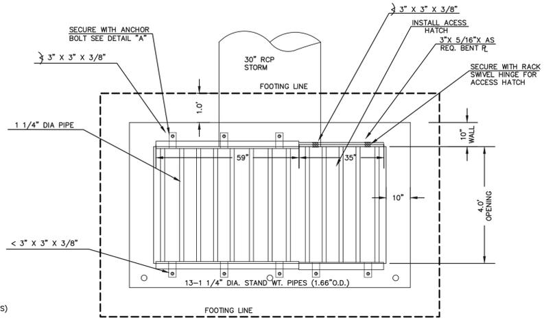
**10'X4' OUTLET BOX OVERFLOW TRASH RACK**
