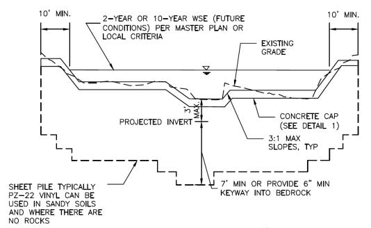
NOTE: THE STRUCTURE MAY BE COVERED WITH 6" OF SOIL OUTSIDE OF THE LOW FLOW AREA.
