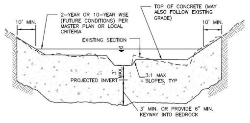
NOTES: 1. TRENCH IN UNDISTURBED SOIL. FORM TOP 6" OF CHECK. DO NOT OVER EXCAVATE TO FORM WALLS OR CONSTRUCT A FOOTING.
