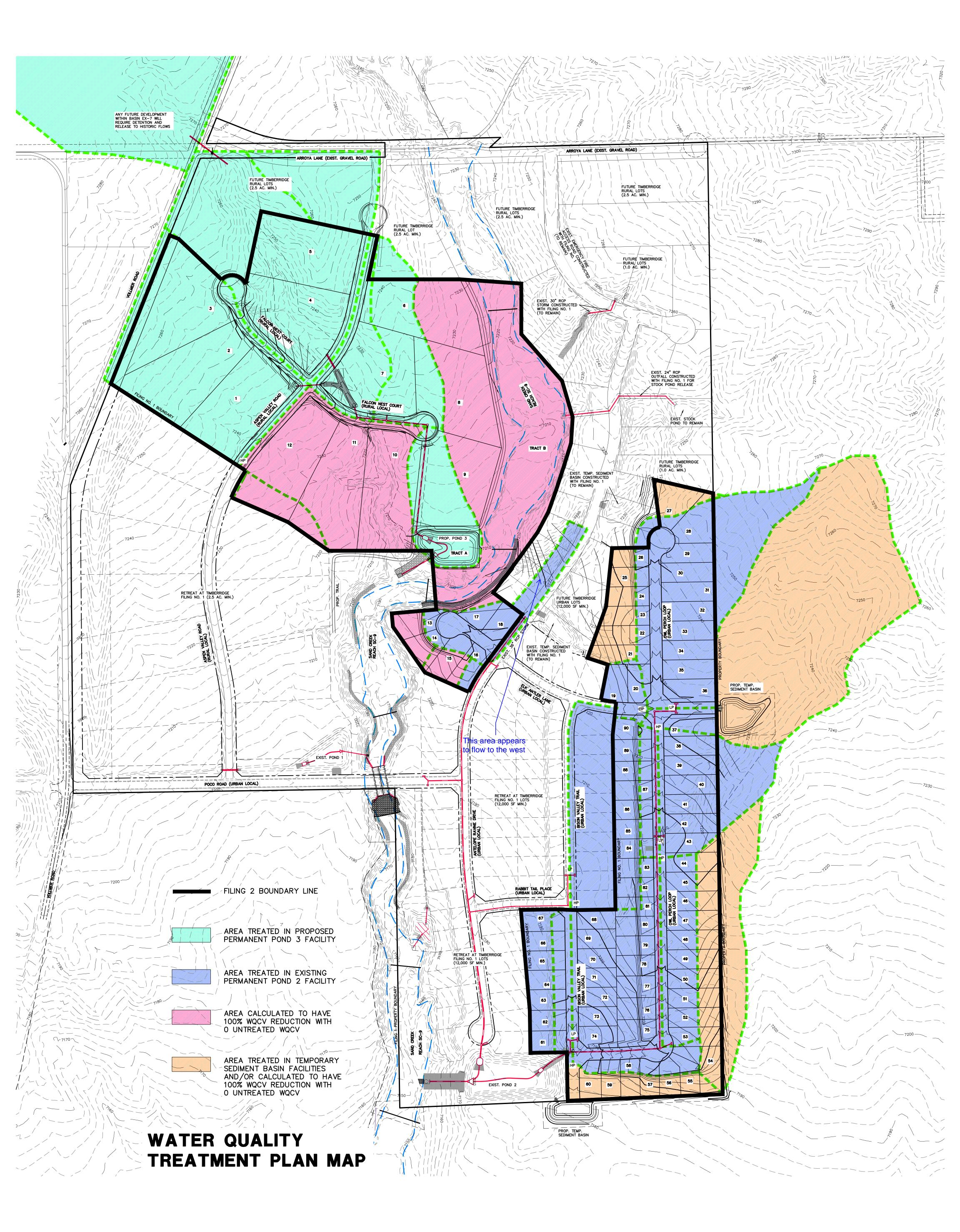
provide a figure showing all proposed UIA and RPA areas to be utilized for runoff reduction. All RPA areas will need to be within a no build/drainage easement and discussed in the maintenance agreement and O&M Manual.
