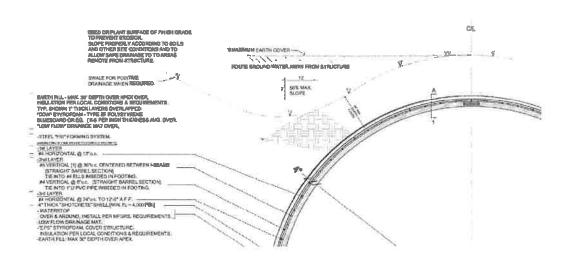
Additionally, the backfill and capping process will have the ground slope limited to less than 58 degrees to prevent erosion or exposure of the structure. Planting cover vegetation while limiting the soil slope to 58DEG or a 7 and 12 pitch and redirection of surface flows will mitigate and prevent excessive erosion.
