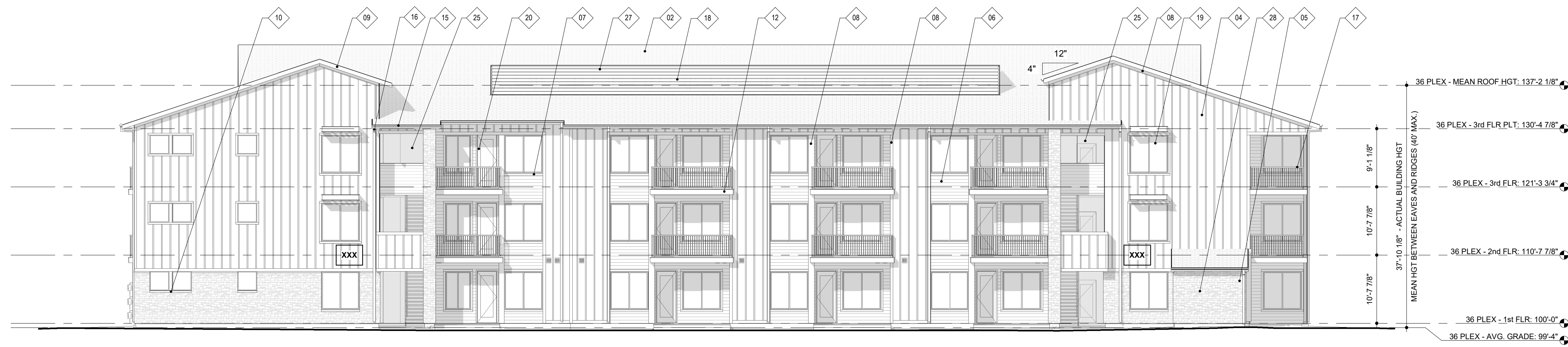
1 BUILDING TYPE A - PLANNING FRONT ELEVATION 3/32" = 1'-0"
