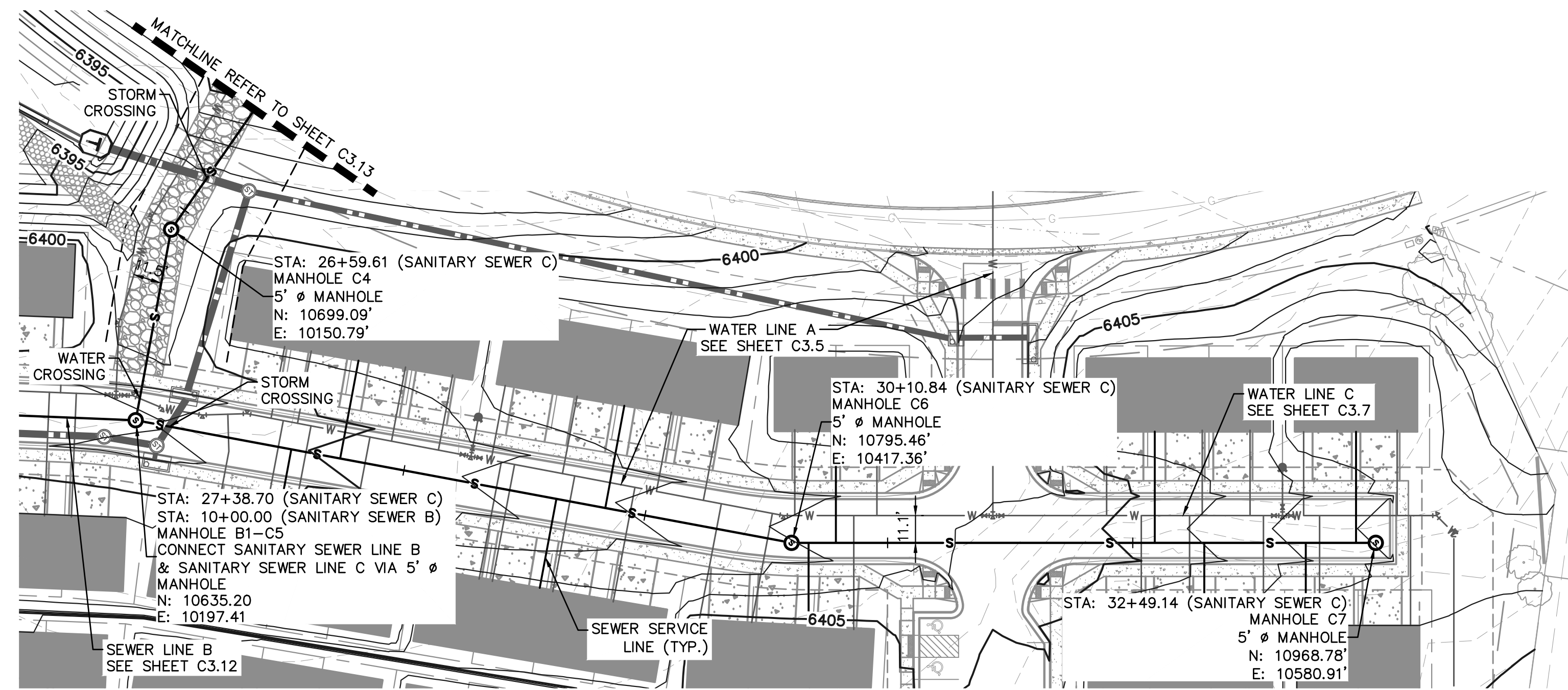
SEWER LINE C STA. 26+00 - END PLAN & PROFILE
