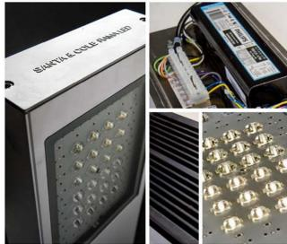
Rama is equipped with Constant Light Output (CLO) technology. CLO programmatically compensates for lumen depreciation by adjusting the drive current, allowing light output to remain constant throughout the luminaire maintenance cycle.
