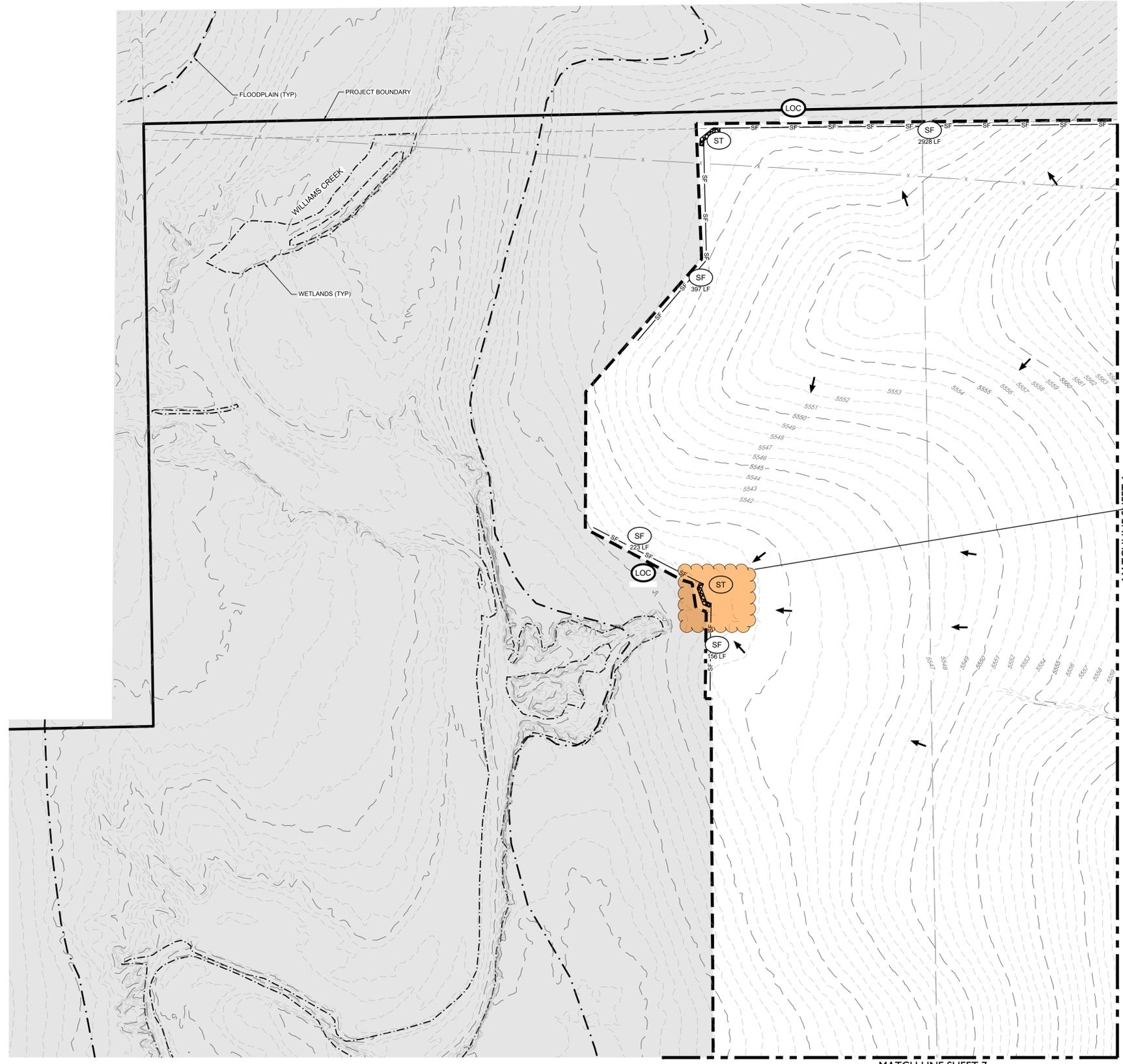
Sediment traps are not appropriate for this application. Temporary sediment basins should be used for tributaries greater than 1 ac. (typ.)
