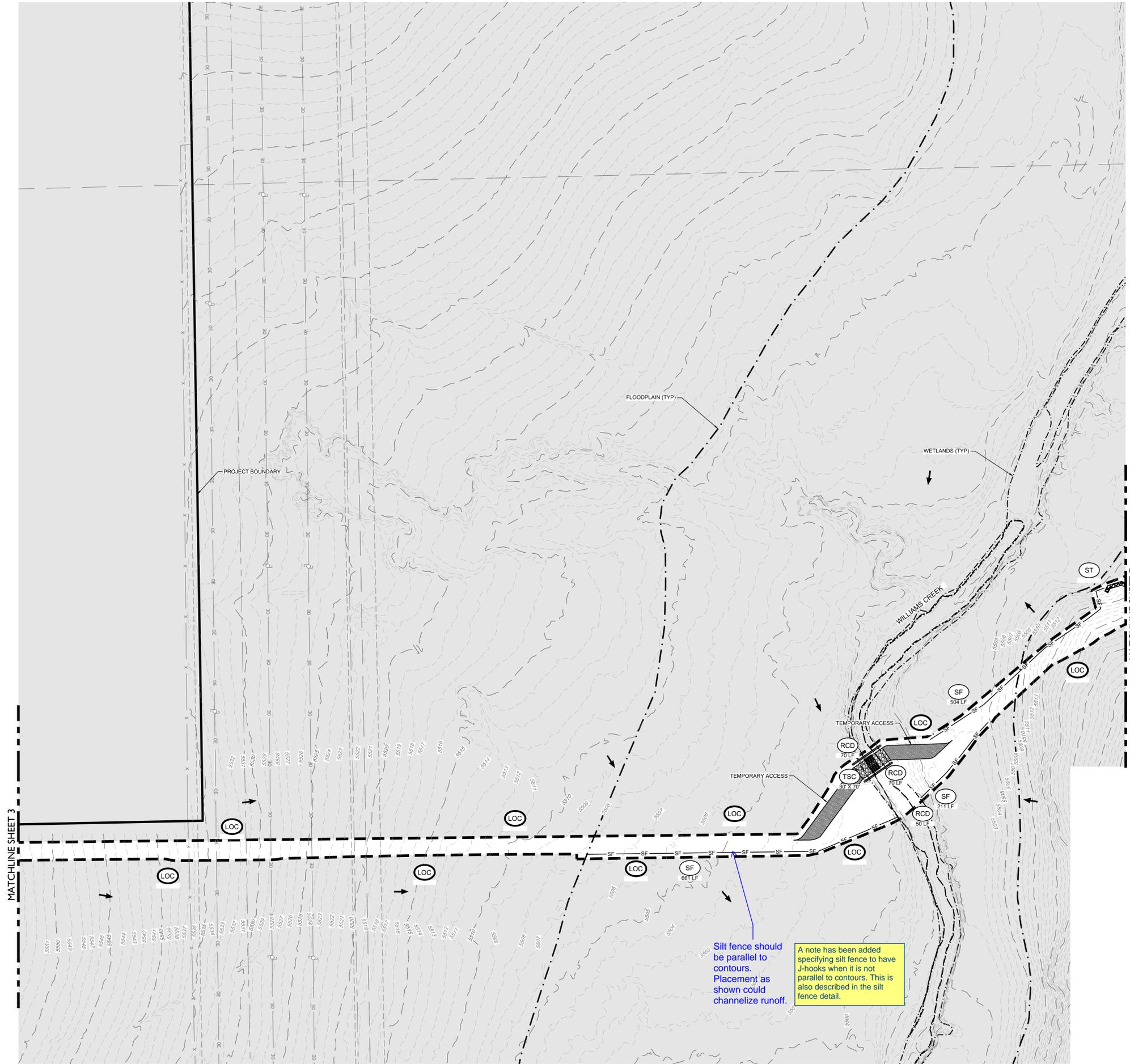
Silt fence should be parallel to contours. Placement as shown could channelize runoff.
