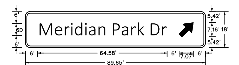
01-1d CIRCULAR INTERSECTION EXIT DESTINATION (1 LINE) 2.25' RADIUS, 0.75' BORDER, WHITE ON GREEN [Meridian Park Dr] 60
