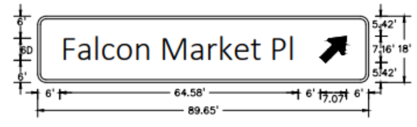
D1-1d CIRCULAR INTERSECTION EXIT DESTINATION (1 LINE) 2.25" RADIUS, 0.75" BORDER, WHITE ON GREEN [Falcon Market Pl] 60
