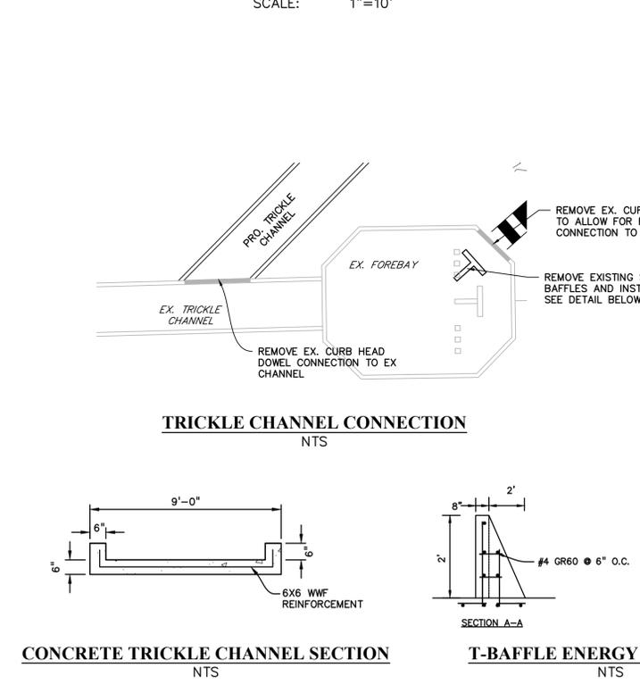
**CONCRETE TRICKLE CHANNEL SECTION**
