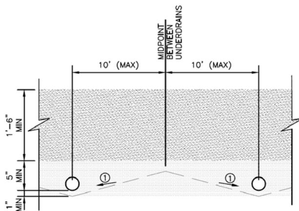
① SLOPE (STRAIGHT GRADE) SUBGRADE (2-10%) TO UNDERDRAIN TO REDUCE SATURATED SOIL CONDITIONS BETWEEN STORM EVENTS (OPTIONAL)
