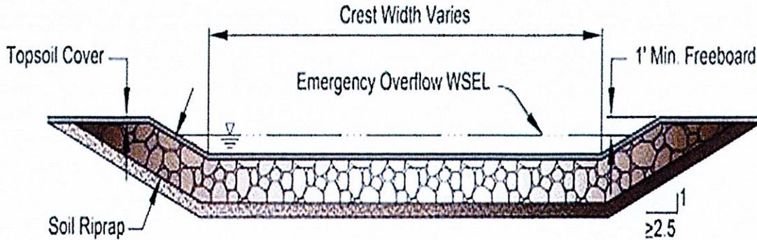
Figure 13-12d. Riprap Types for Emergency Spillway Protection
