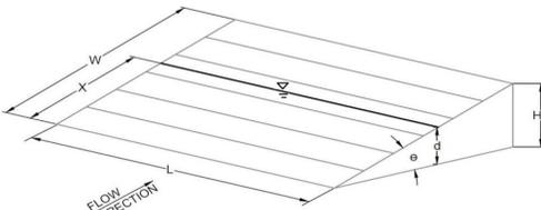
Water Depth at Inlet (for depressed inlets, 1 foot is added for depression)
