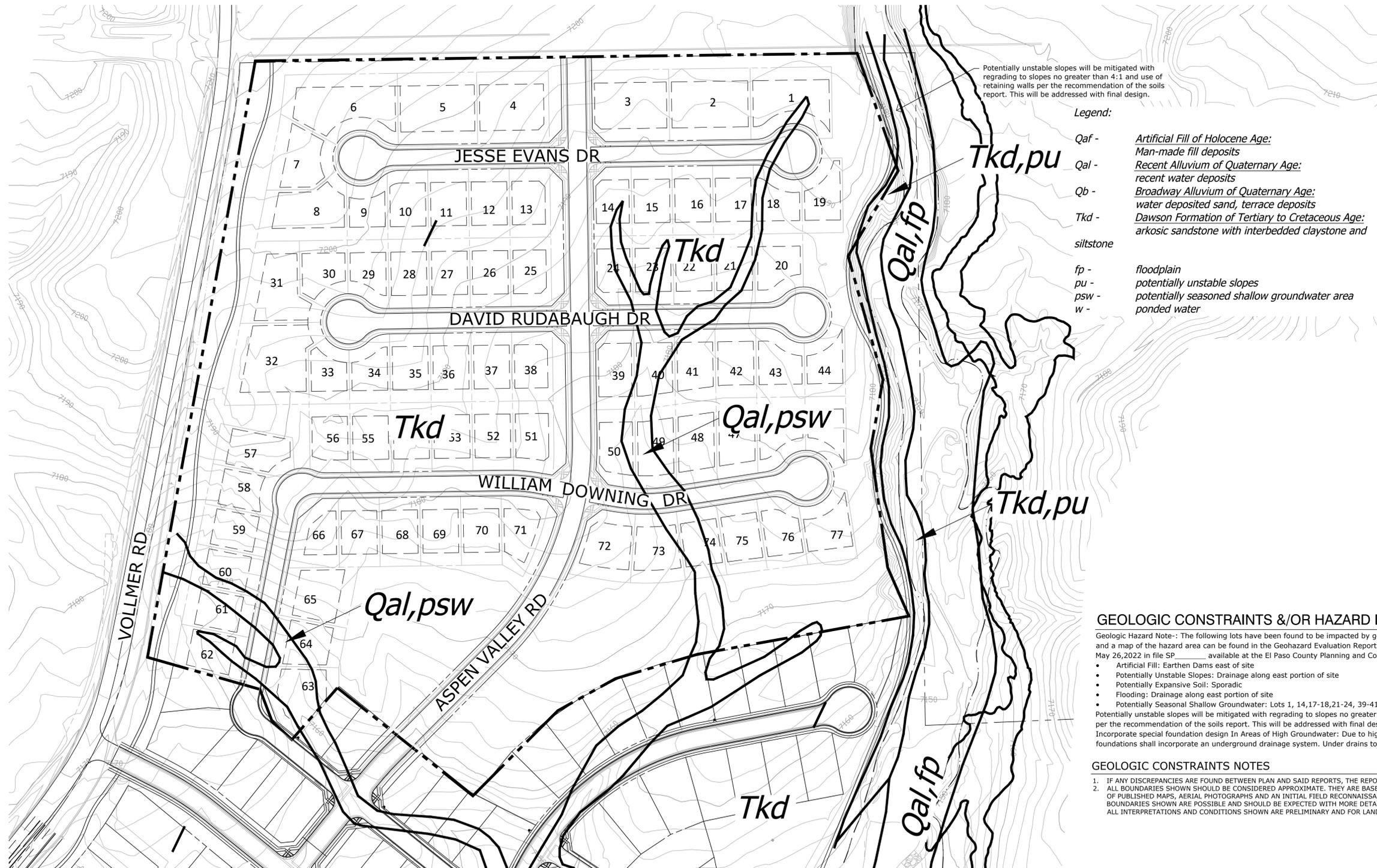
Potentially unstable slopes will be mitigated with regrading to slopes no greater than 4:1 and use of retaining walls per the recommendation of the soils report. This will be addressed with final design.
