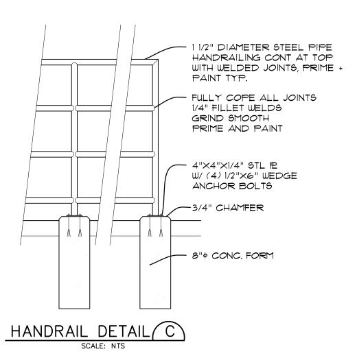
PROVIDE HANDRAIL ALONG ALL RETAINING WALLS & DRAINAGE STRUCTURES WITH OVER 30" HEIGHT ABOVE GRADE
