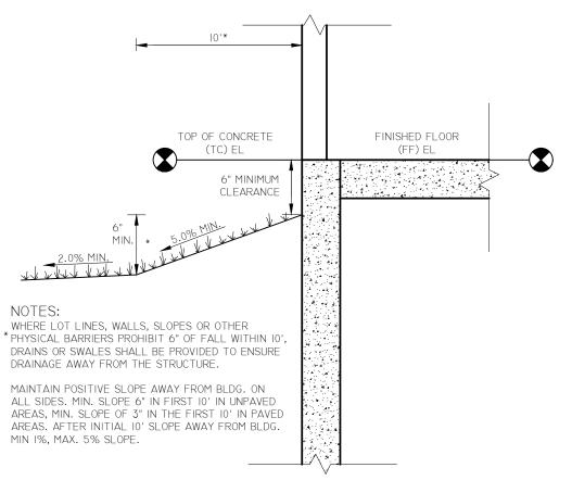
TYPICAL BUILDING DRAINAGE DETAIL 3
