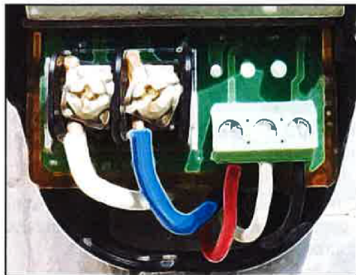
Ped Call Terminal on left. 3-position terminal block on right (for operating as iNS3)
