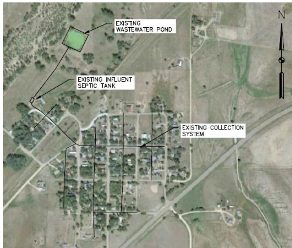
Figure 3 – Existing Facility Aerial
