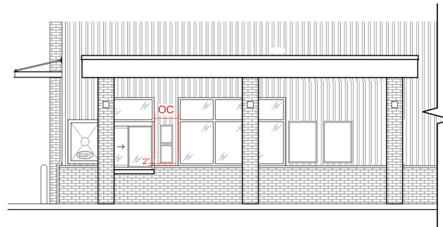
(UNLESS OTHERWISE DIRECTED) CENTERED BETWEEN MULLIONS 2" ABOVE STONE CAP 1" VERTICAL GAP BETWEEN SNAP FRAMES
