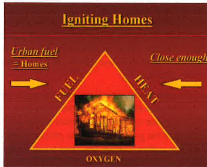
Figure C-2-1. Homes ignite and burn during wildfires when the requirements for combustion, a sufficiency of fuel, heat, and oxygen are sustained at one or more places on a home. The amount of heat transfer depends upon the fire's intensity, its distance from the home, and the duration (time) of the exposure.
