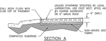
VTC-1. AGGREGATE VEHICLE TRACKING CONTROL
