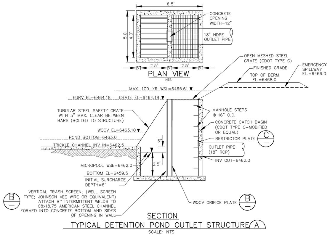
**VERTICAL TRASH SCREEN:** (WELL SCREEN TYPE; JOHNSON VEE WIRE OR EQUIVALENT) ATTACH BY INTERMITTENT WELDS TO C8x18.75 AMERICAN STEEL CHANNEL FORMED INTO CONCRETE BOTTOM AND SIDES OF OPENING IN WALL
