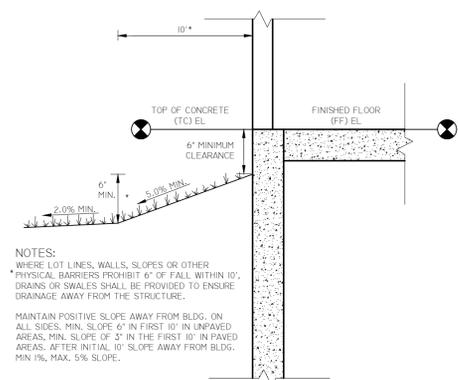
TYPICAL BUILDING DRAINAGE DETAIL (3)
